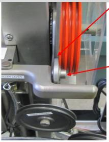
Alignment of Pressure Roller to the center of the first groove in the lower capstan should be adjusted if found to be 'off center'.
